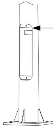
The beam in the service hatch is required to hang HCU on it.
