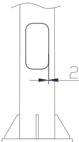
Option 2. Drill a  $\phi 25$  hole on the door and attach a cover over it in case of rain ingress.
