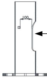
The service hatch must be more than 300mm X 100mm
