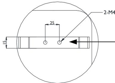
A beam in the service hatch is required with two M4 screw holes drilled into it.
