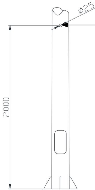
A hole (at least  $\phi 25$  mm) must be drilled 2 meters from the bottom of the pole and attached with a cover to avoid rain ingress, as shown in the picture.
